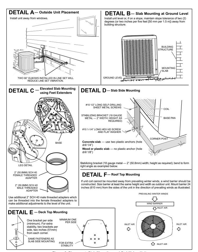
Figure 6. Placement, Slab Mounting and Stabilizing Unit
